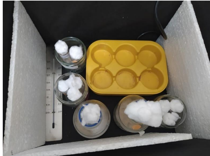
Fig. 29. Carton box with yogurt maker and foam core boards on the sides. A thermometer is used to check the temperature (own source).
