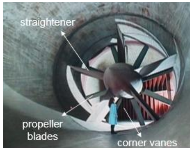
Driver section: low-speed wind tunnel CIA-IUA (Argentina)
