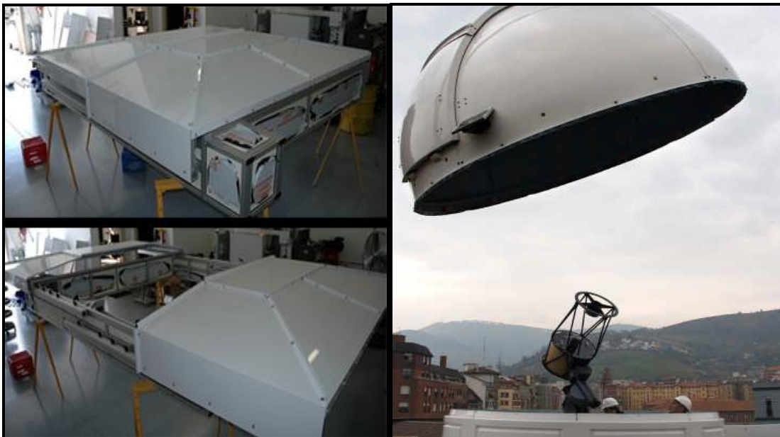
Sostre corredís (roll-off-roof)
