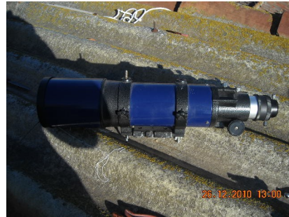
Refractor 500mm focal
