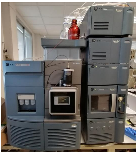
Figura 27. Cromatograf UPLC aoblat a un detector de masses tipus triple quadripol model Xevo TQS.
