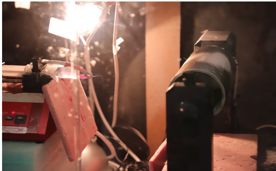
FIGURE F.20. This is the electrospinning method.
