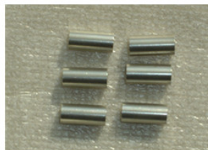
FIGURE 2.4. Example of alloy made of chromium (Cr), cobalt (Co) and molybdenum (Mo).
