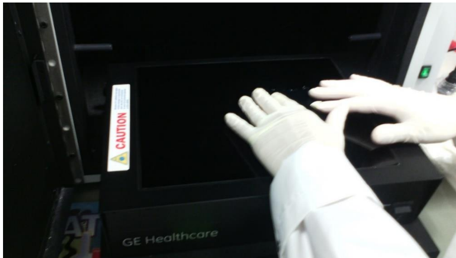
Figure 32. Process of placing our DNA gels to the dark chamber. The dark chamber provides darkness, so UV lights don't have any type of interference and our samples can be monitored. (Own authorship)
