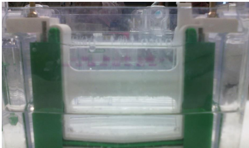
Figure 31. Migration of the DNA samples. After the samples are loaded into the wells, voltage is applied so our negative samples can migrate towards the positive pole. (Own authorship)
