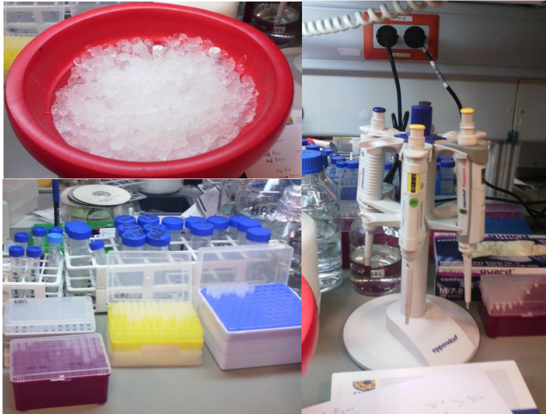
Figure 25. Materials used for the phosphorylation process. At the top left, an ice bucket to conserve our DNA samples. At the bottom left, micropipette tips with different sizes depending on the quantity that we have to take. At the right, micropipettes, measurement instruments used for taking small quantities (from 0,1 \mu\text{l} to 200 \mu\text{l} ) of our samples. Each micropipette has got a corresponding tip to work with. (Own authorship)
