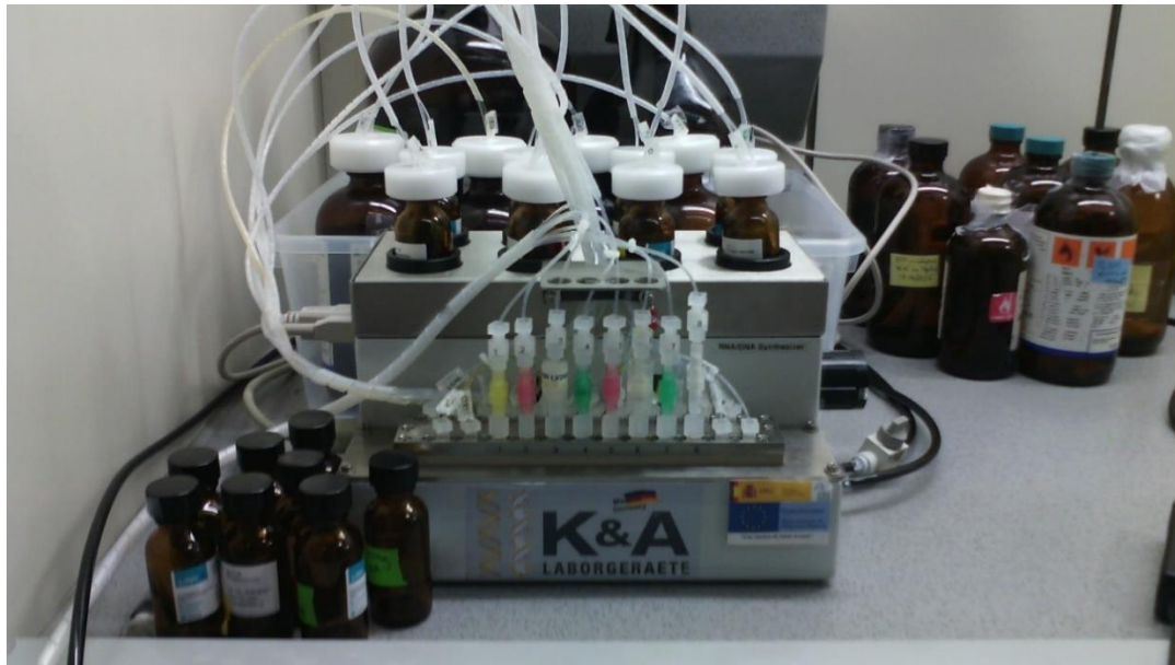
Figure 10. DNA synthesiser. This machine is used to synthesise DNA chains. Each of the tubes contain a different ribose. Each nucleoside is added following the Phosphoramidite Method. This procedure is repeated as many times as needed by introducing a command to the computer that controls the synthesiser. (Own authorship)
