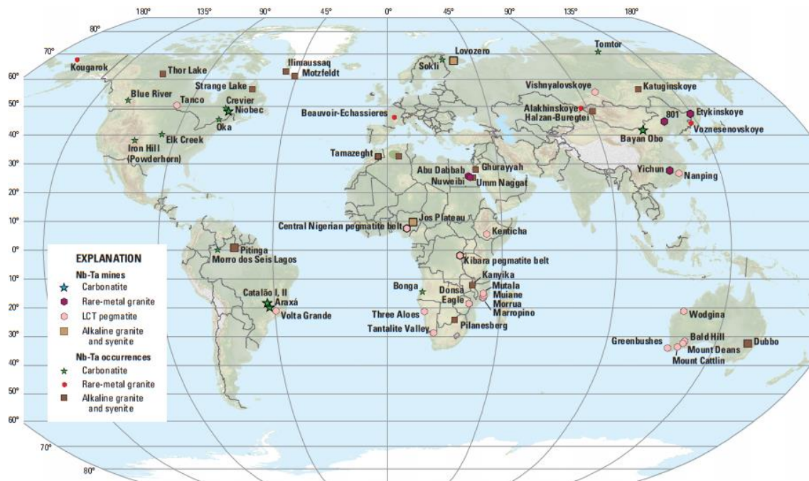
Figure M5. World map showing locations of selected niobium and tantalum mines, deposits, and occurrences, by deposit type. Not all the mines are currently active. LCT, lithium-cesium-tantalum; Nb, niobium; Ta, tantalum
